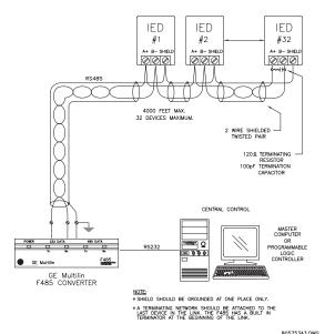
Figure 1: RS232 to RS485 connection
